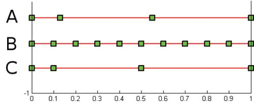
**Fig. 7.** Lookup table positions representing the universe of discourse in an antecedent dimension. A: input points, B: universe with a fixed resolution, C: input points aligned to the positions of the universe.
