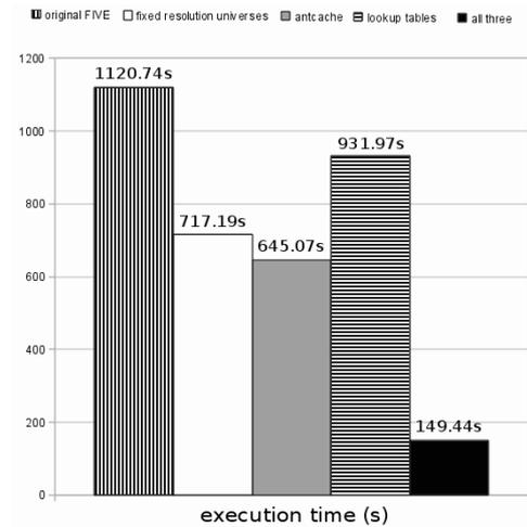
**Fig. 8.** Execution times of the vehicle navigation application benchmark, from left to right: unmodified FIVE, FIVE with fixed resolution universes, FIVE with antecedent caching, FIVE with conclusion lookup tables, and FIVE with all the modifications.
