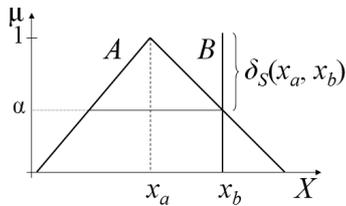
**Fig. 1.** The  $\alpha$ -cuts of  $\mu_A(x)$  contain the elements that are  $(1 - \alpha)$ -indistinguishable from  $x_a$ , where  $A$  is a fuzzy set and  $B$  is a singleton fuzzy set at  $x_b$ .
