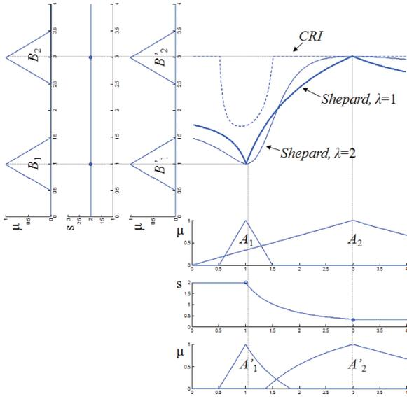
**Fig. 4.** Interpolation of two fuzzy rules ( $R_i : A_i \rightarrow B_i$ ), using the Shepard-operator-based FIVE (“Shepard” (3)), and for comparison, the min-max CRI with “center of gravity” defuzzification (“CRI” on figure).
